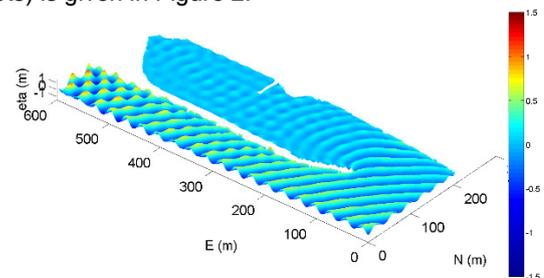
Figure 2 - Instantaneous sea surface elevations for the alternative layout A-1. Ship waves  $T=4$  s ( $V_k=12.2$  knots).
