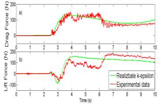
Figure 4 - Comparison between numerical model (Realizable k-epsilon turbulence model) and experimental data. Dry bed condition, h=50cm, e/D=0.6. a) Drag force time history,  $R^2$ =0.8 b) Lift force time history,  $R^2$ =0.6.
