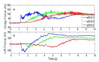
Figure 2 - Time-history of the a) drag force b) lift force for drybed condition, h=40cm, e/D=0.3,0.6,0.8.
