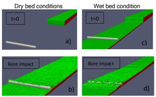
Figure 3 - 3D view of OpenFoam CFD model, a & b) Dry bed condition. c & d) Wet bed condition.
