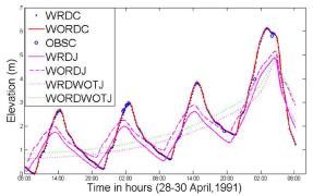
Figure 1 - Water level due to the April 1991 cyclone, WRDC indicates Water level with river discharge effect at the Coxbazar tide station. Similarly, Water level without river discharge (WORDC),Observed (OBSC), Water level with river discharge at Junction point (WRDJ), Water level without river discharge(WORDJ), Water level with river discharge at Junction point without tide(WRDWOTJ), Water level without river discharge and without tide(WORDWOTJ)
