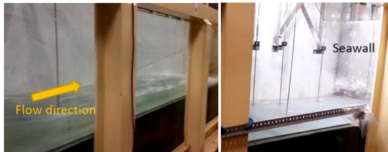
Run-up test Wave pressure test Figure 7. Examples of hydraulic flume tests for wave run-up and pressure.
