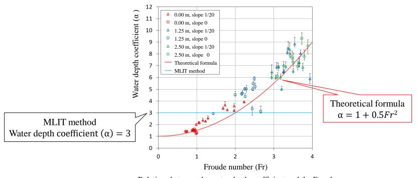
Relations between the water depth coefficient and the Froude number when the specific energy becomes the maximum
