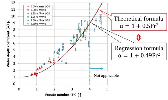
Relations between the water depth coefficient and the Froude number when the specific energy becomes the maximum
