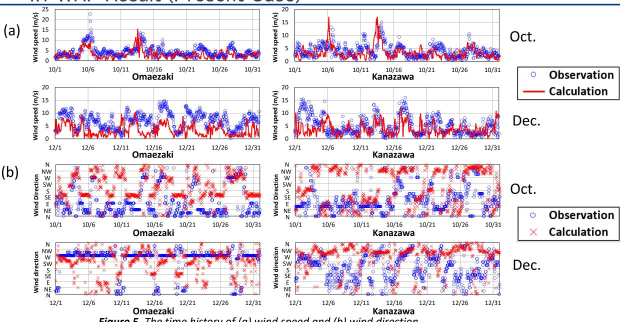
Figure 5. The time history of (a) wind speed and (b) wind direction
