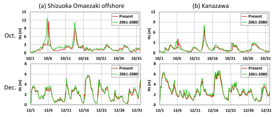
*Figure 9.* Comparison of the time history of significant wave height between present and future case
