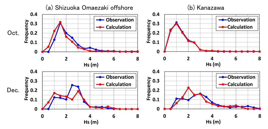
*Figure 7.* The frequency distribution of significant wave height
