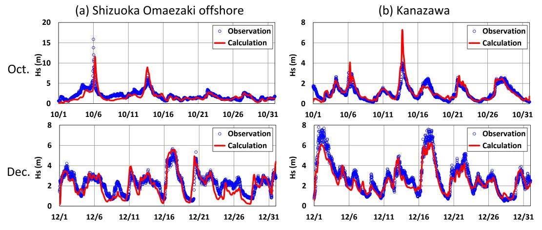
*Figure 6.* Comparison of the time history of significant wave height
