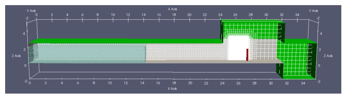
OpenFOAM (Open source Field Operation And Manipulation) Solver: InterFoam based on the volume of fluid (VOF) method Mesh size:  $\Delta x=12.5$ cm (upstream), 1.56 cm (near the vertical wall) Turbulence model: LES Smagorinsky Boundary conditions: No-slip (floor, side wall, the vertical wall)
