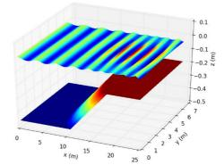
Figure 1 - Bathymetry of the experiments of Whalin (1971) and snapshot of the simulated free surface elevation.
