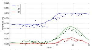
Figure 2 - Simulated (solid line) and measured (dots) harmonic amplitudes along the center axis of the basin for an experiment of Whalin (1971) with T = 2 s and A = 7.5 mm.
