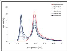
Figure 3: A snapshot of differently partitioned percentages of Swell energy built-up observed in St. Mary Sound at different dates in December 2014 (CCO, 2017).
