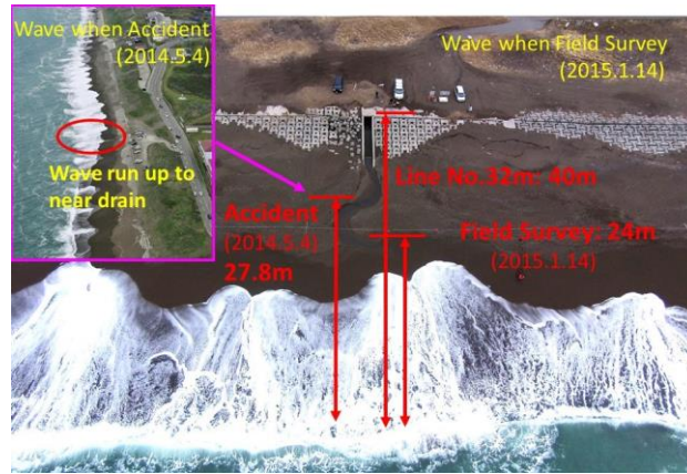
Figure 2. Compare Distance of Wave Run Up at Accident Date and Field Survey Date.
