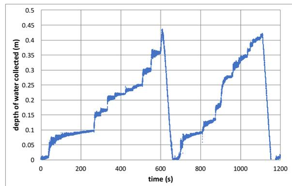
Figure 5: Example overtopping collection tank depth vs. time data. Test 5.6; swell normal; sea obliquity =  $60^\circ$ .
