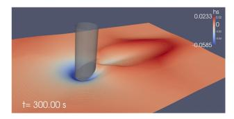
Figure 2 - Bed elevation after 300s of dynamics.
