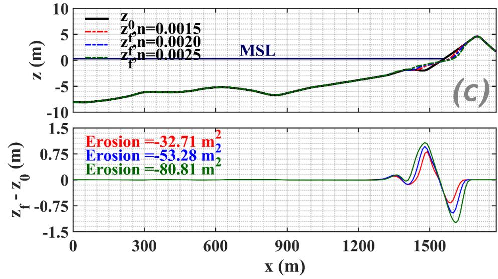
CSHORE a) Grid b) Breaker Index c) Bed Friction Sensitivity
