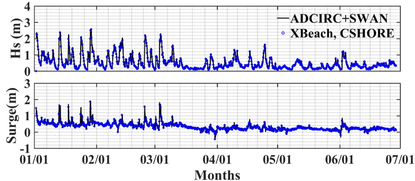
*Water Level & Wave Height at Offshore Boundary of P1 to P5 in XBeach & CSHORE*
