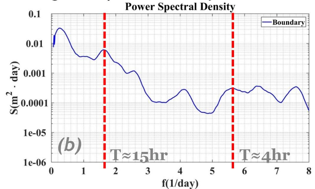
Power Spectral Density (PSD) of hourly water level at a) Stations 9063020 & 9063028 b) Boundary of Profiles P1-P5 for selected time window.
