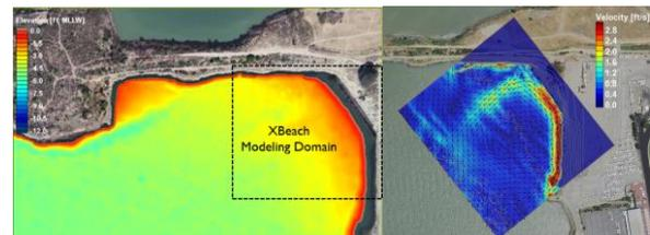
Figure 1 - Project site bathymetry and features, and XBEACH modeling domain (left), and nearshore wave-generated currents from XBEACH (right).
