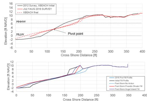
Figure 2 - Measured and reproduced beach profile changes at center of pocket beach (top), and beach profile adjustments through estimated four (4) years of storm activity for three beach nourishment material alternatives (bottom).
