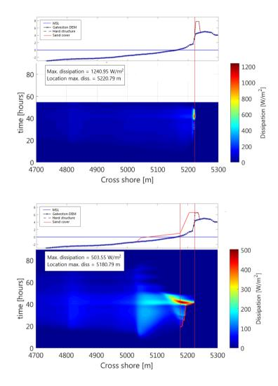
Figure 9. Characteristic cross-section and cross-shore wave dissipation timestack for the reference case (upper panel) and hybrid design with Run ID 2.10 (lower panel). The reference case was stopped at 55 hours as maximum dissipation had passed. Indicated by the red line is the location of either the dune face or the toe of the seawall once exposed for retrieving the maximum wave height at the face of the hybrid structure.
