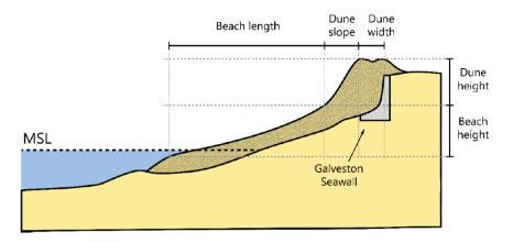
Figure 3. Schematic cross-section of the hybrid setup under consideration. Design parameters that were varied as part of this study are displayed.
