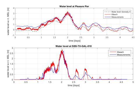
Figure 7. Storm surge validation between predicted (red) and measured (blue) water levels for the Galveston Pleasure Pier tidal gauge (SID: 8771510; 29°17.1 N; 94°47.3'W (NOAA, 2016c)) in front of the GSW (top panel) and at a temporary onland gauge (SID: SSS-TX-GAL-010; 29°14.1'N 94°52.4'W (USGS, 2008)) at the west end of the GSW, where only small dunes are present (bottom panel).
