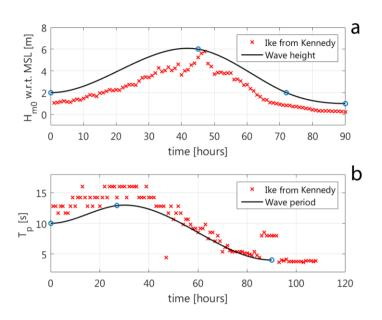
Figure 6. Time series of design significant wave height (a) and peak wave period (b) used for the hybrid simulations (black). Reference is made to the measured wave height and period during Hurricane lke by rapidly deployed buoys in around 10 m water depth along the Upper Texas Coast (Kennedy et al., 2011a).
