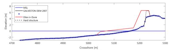
Figure 4. Cross-section of hybrid setup for simulation with run ID 2.10 (see Table 1). In this case GSW is increased to MSL + 6.5 m.
