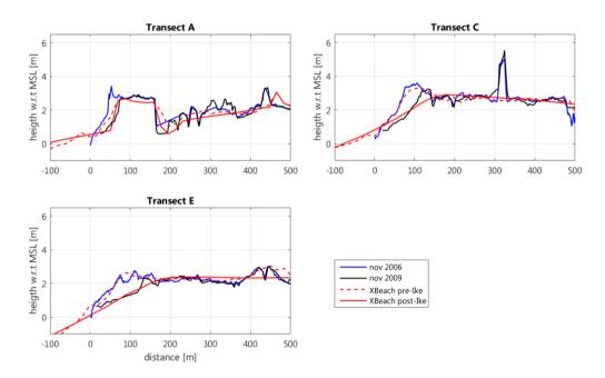
Figure 8. Predicted and measured cross-shore profiles before and after Hurricane lke impact at the west end of the GSW on Galveston Island. Transect A is located just west of the west end of the GSW and features several non-erodible structures, such as a parking lot and elevated roads. Transects C and E are located westward of transect A and feature only small dune formations. The large elevation in the middle of Transect C represents a man-made structure and was not included in the model.
