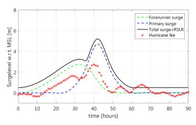
Figure 5. Time series of storm surge level for a 100-year event including forerunner surge (green) and primary surge (blue) (Lendering et al., 2014) and final combined surge level accounting for RSLR (black). Reference is made to measured surge levels during Hurricane Ike at offshore buoy S42035 (NOAA, 2016a).
