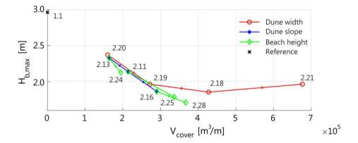
Figure 10. Wave height at the face of the hybrid structure versus the volume of sand material covering the structure. An overview of the design parameters for the displayed cases can be found in Table 1.
