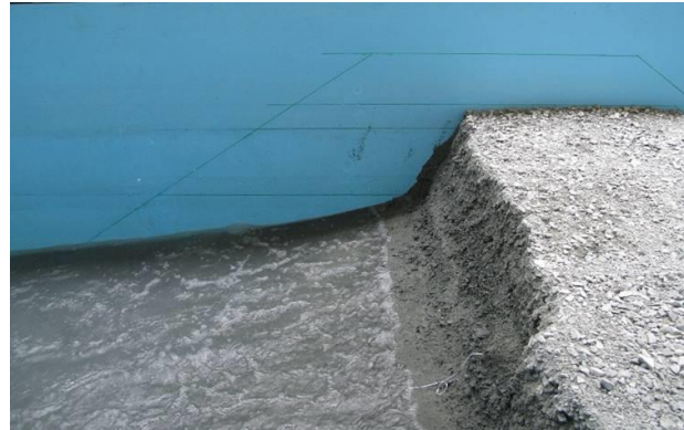
Figure 1 - Typical damage profile of emerged gravel bund from physical model test
