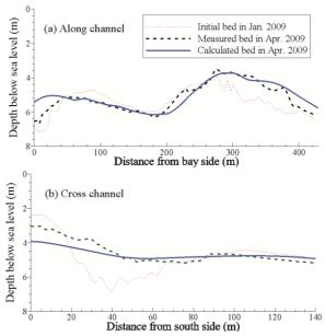
Figure 2 - Measured vs. Calculated Bed Levels
