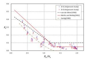
Figure 2 - Test results for transmission coefficient and comparison with previous results : the effect of width of superstructure (B)
