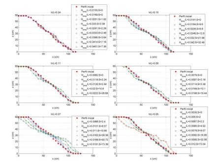
Evolution of the profile depending on the wave slope, the incoming wave train and the typology
