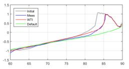
Figure 2. Measured and simulated beach profiles under a storm wave condition (Hs=1.17 m, Tp=4.90 s, d =4.13 m)
