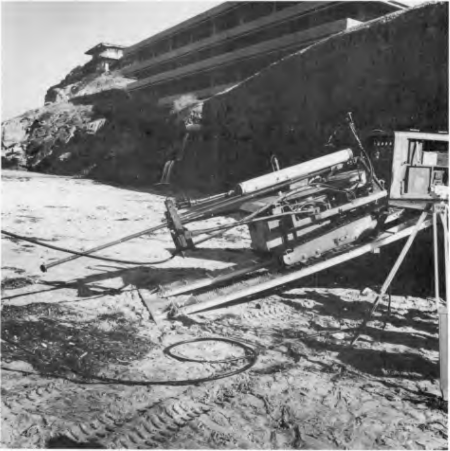
PROFILER DESCENDING FROM TRANSPORT VEHICLE PRIOR TO BEACH SURVEY. THE PROFILER WILL BE TURNED THROUGH 180° BEFORE BEGINNING A RUN.
