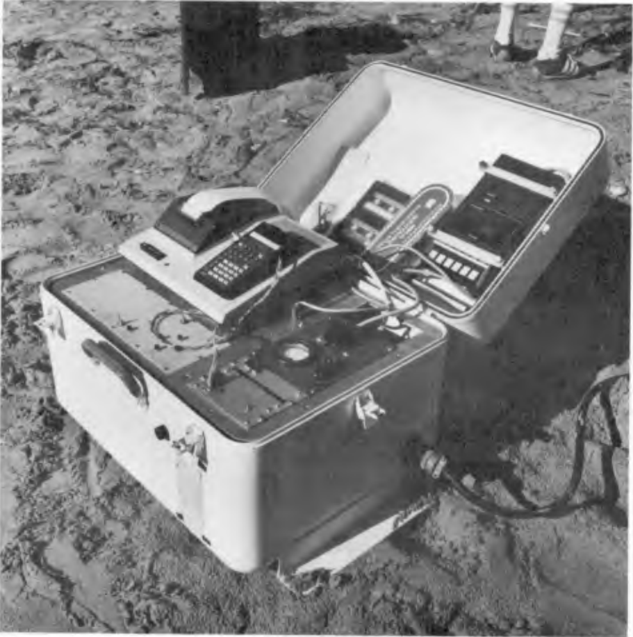
THE PROFILER CONTROL CONSOLE CONTAINS TRACTOR DIRECTIONAL CONTROLS, A PLOTTER FOR POSITION VISUALIZATION, THE DATA RECORDER AND INSTRUMENT STATUS CHECKOUT EQUIPMENT.
