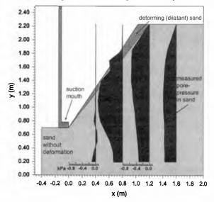
Figure 12: Pore pressure changes in front of suction mouth.
