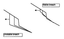
Figure 4: Stable and Unstable breaching.
