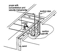
Figure 7: Set-up of the model experiments.
