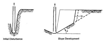
Figure 2: Slope development resulting after sudden disturbance.
