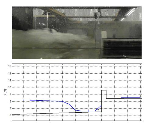
Figure 15. One example of snap shot of wave tip in front of the dike from physical model and SWASH model.
