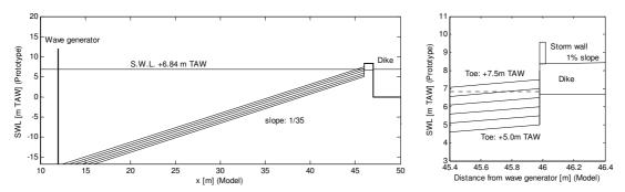
Figure 3. Numerical experiment setup for different beach levels. Left shows the entire figure and right is a close up of at the dike.
