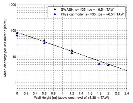
Figure 2. Numerical model and physical model for mean wave overtopping discharge against different storm wall height.
