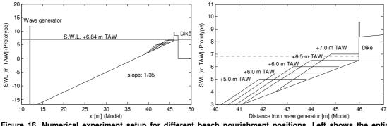
Figure 16. Numerical experiment setup for different beach nourishment positions. Left shows the entire figure and right shows near the dike.
