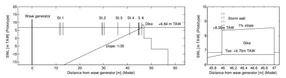
Figure 1. Experimental setup of wave transformation and wave overtopping on the Wenduine sea dike (SWL=6.84 m TAW, 1:25 scale)
