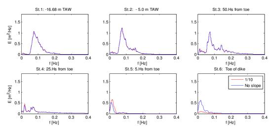
Figure 12. Comparison between 1/10 slope and no slope for the wave energy spectrum at each station.
