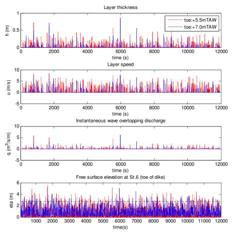
Figure 8. Comparison between the toe level of +5.5 m and +7.0 m TAW for the time series of layer speed, velocity, discharge and free surface elevation.
