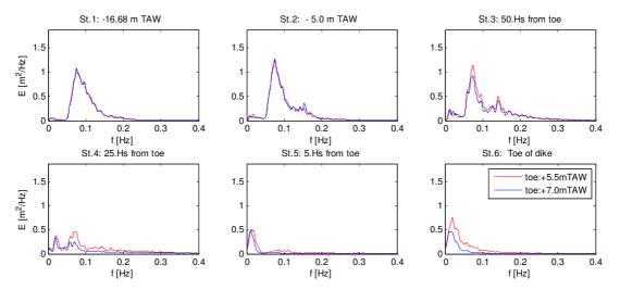
Figure 6. Comparison between the toe level of +5.5 m and +7.0 m TAW for the wave energy spectrum at each station.
