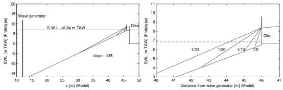
Figure 9. Configuration of beach slopes for 1/5, 1/10, 1/20 and 1/30. Left shows the entire domain and right shows near the dike. Toe level, dike crest and wall crest level are +6.50 m TAW, +8.38 m TAW and +9.58 m TAW, respectively.
