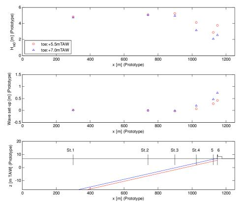
Figure 5. Comparison between the toe level of +5.5 m and +7.0 m TAW for the spatial distribution of Hm0 and wave set-up.
