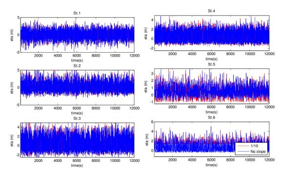
Figure 13. Comparison between 1/10 slope and no slope for the time series of free-surface elevation at each station.
