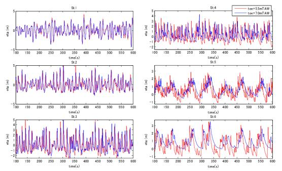
Figure 7. Comparison between the toe level of +5.5 m and +7.0 m TAW for the time series of free-surface elevation at each station.
