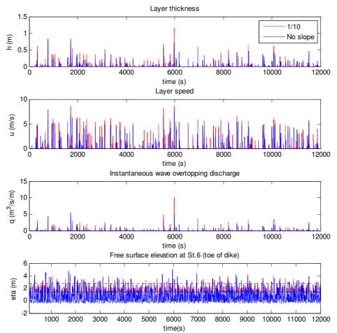
Figure 14. Comparison between 1/10 slope and no slope for the time series of layer thickness, velocity, discharge and free-surface elevation.
