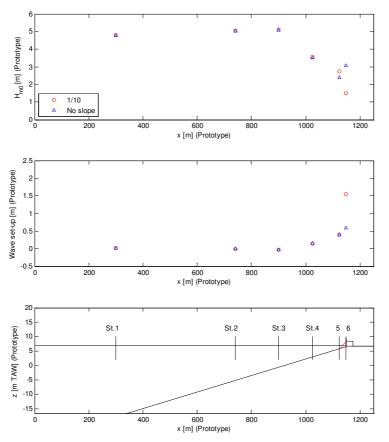
Figure 11. Comparison between 1/10 slope and no slope for the spatial distribution of H<sub>m0</sub> and wave set-up.
